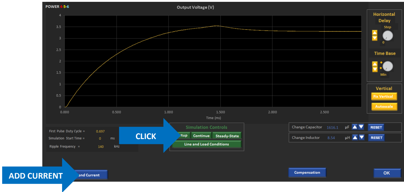
Fig. 2.8: POWER 4-5-6 Start Up Simulation Voltage Waveform
