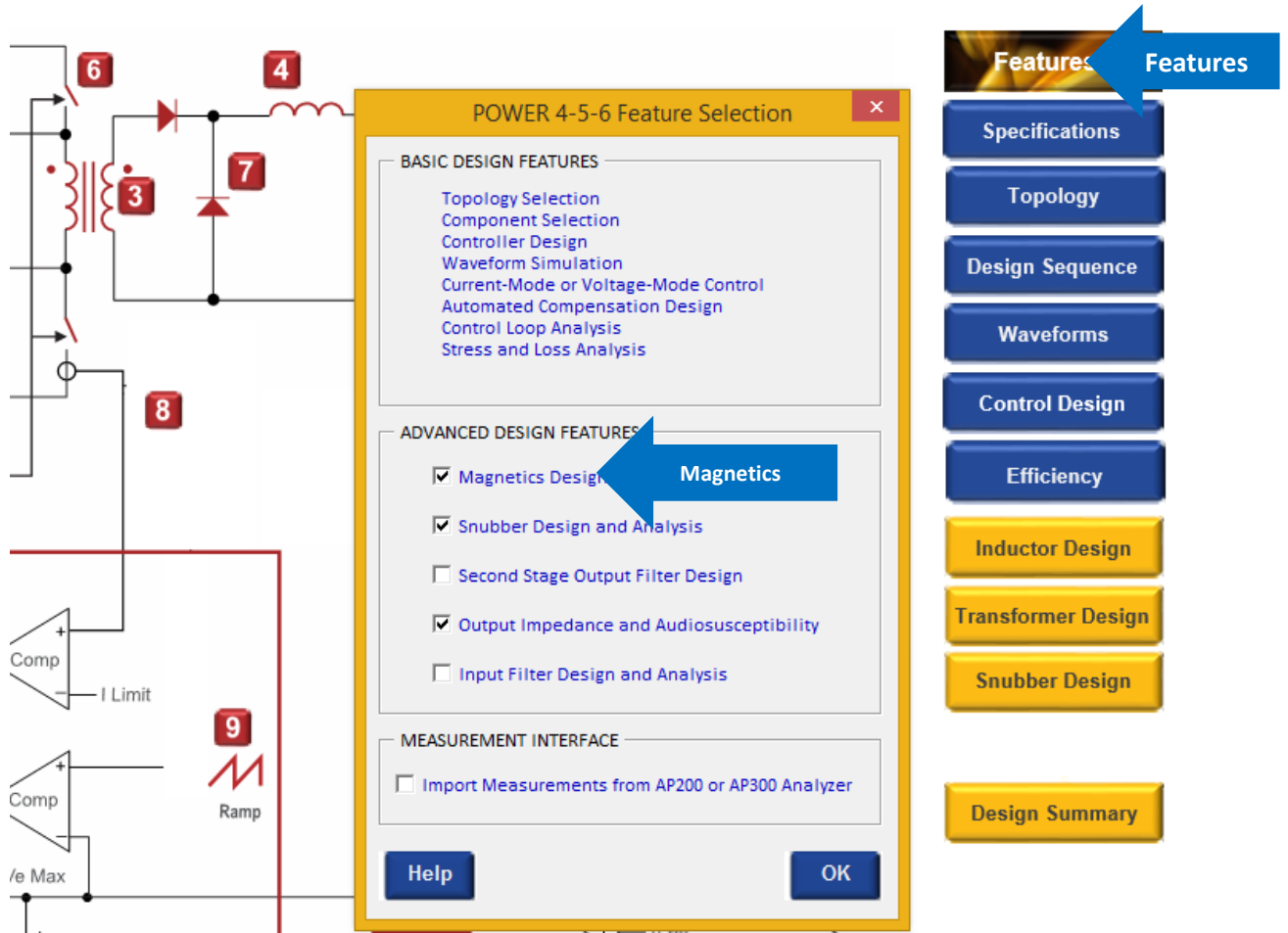
Fig. 4.1: Selecting the Magnetics Design Option Enables the Inductor and Transformer Designers
