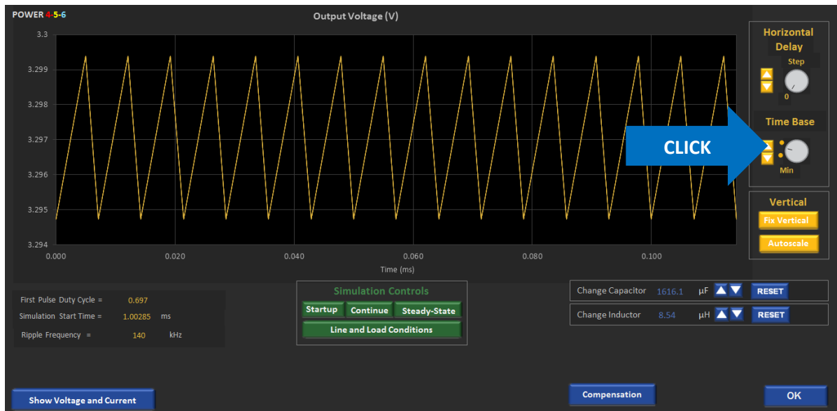
Fig. 2.7: POWER 4-5-6 Expanded Output Voltage Waveform
