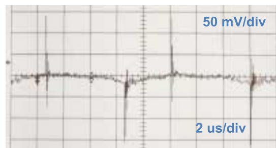
4(a) Conventional 100 kHz PWM Forward
