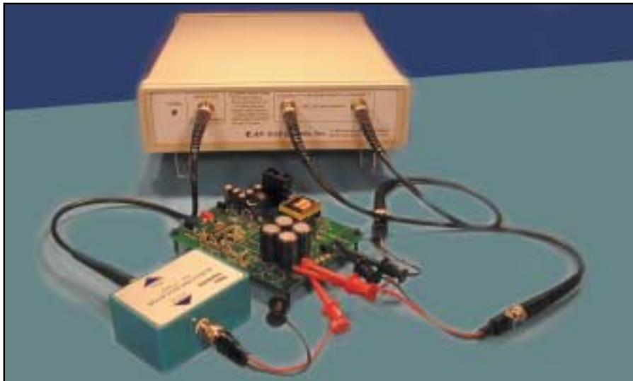
Figure 9a: Frequency Response Analyzer Ready to Measure Loop Gain of a Power Supply
