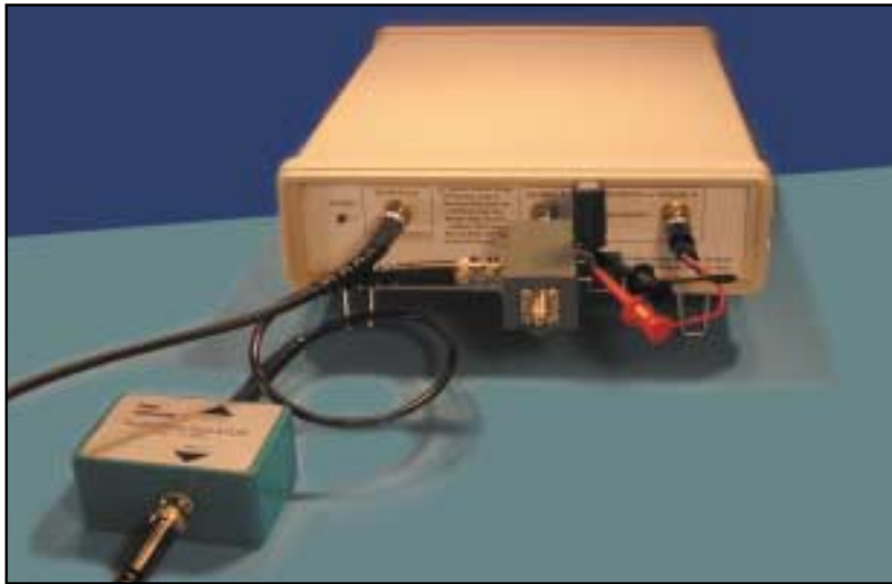
Figure 4a: AP200 Frequency Response Analyzer Ready for Low-Impedance Measurement
