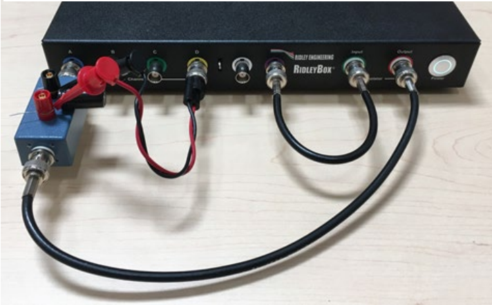
Fig. 6.5: Low Impedance Measurement Setup
