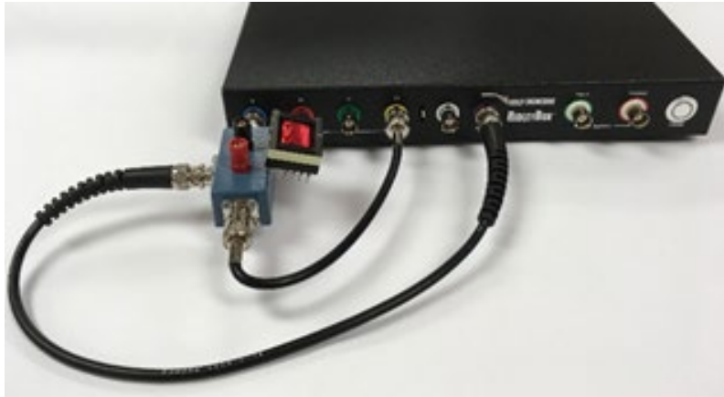
Fig. 6.1: High Impedance Measurements (> 0.1 Ohm)
