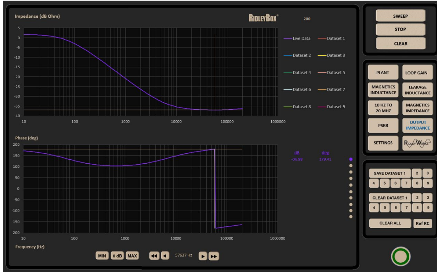
Fig. 7.2: Sweeping the Power Stage Output Impedance
