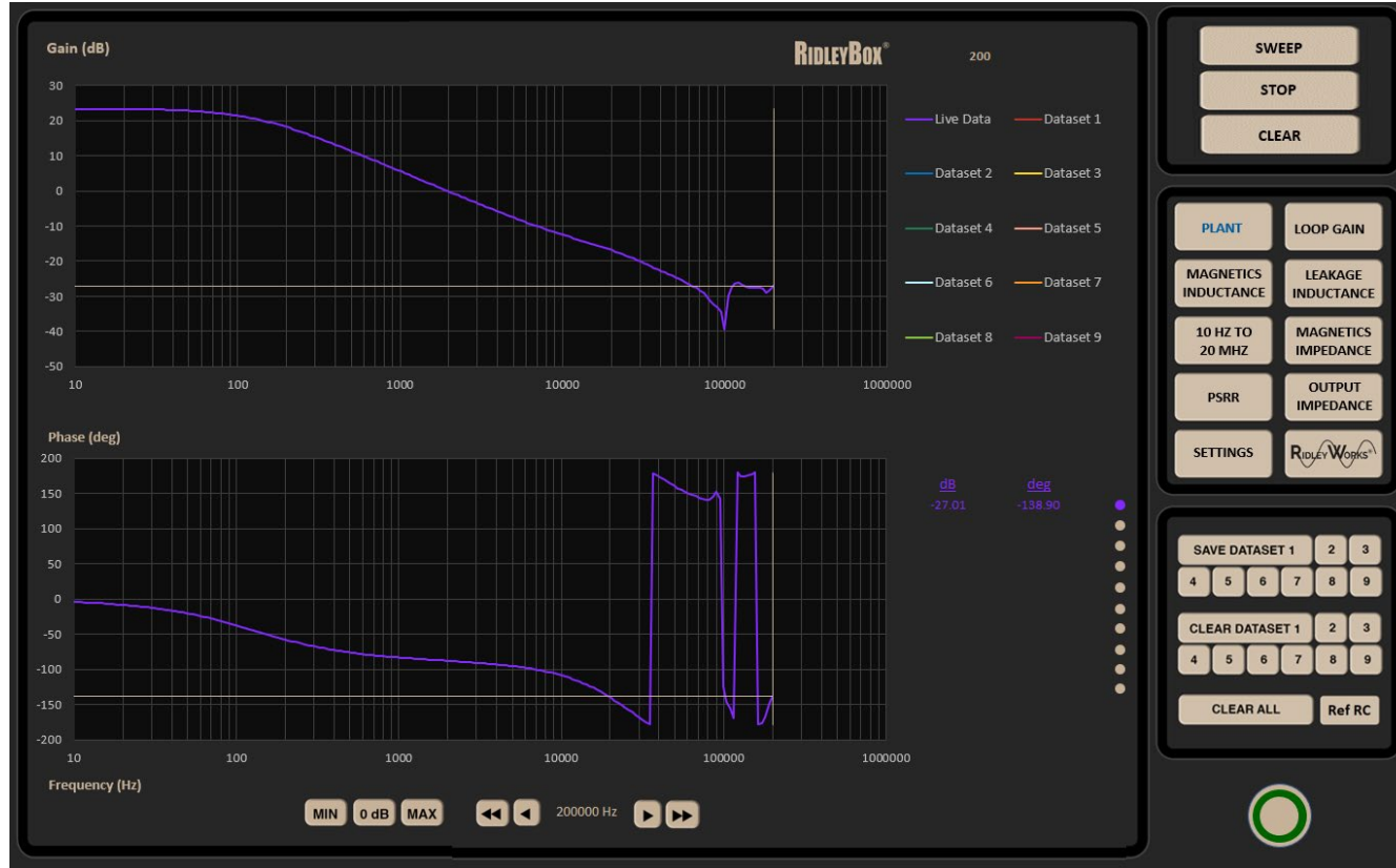
Fig. 5.3: Sweeping the Power Stage
